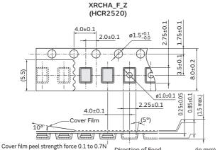
Direction of Feed (in mm) Cover film peel speed 300mm/min.
