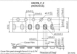
Direction of Feed Cover film peel speed 300mm/min.
